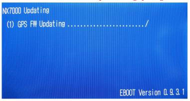
If the screen shows "Retry" or "Fail", press the reset button. After the unit restarts, ejects the SD card and try again. If you have any operational questions or issues after this update, please contact JVC Service Center.
