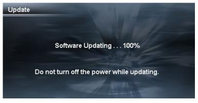
2-13. When update is completed, display changes as shown below. Touch [OK] and the front panel opens.
