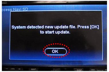
2-11. Display changes as shown below during updating of GPS software. Attention: Do not turn off the power during updating.
